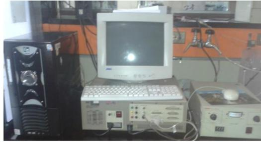
**Figura 16.** Potenciostato/Galvanostato Bass 100<sup>a</sup>.
